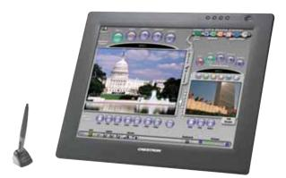
Viewing Angle: ±70° horizontal, ±70° vertical Touchscreen: Resistive membrane
